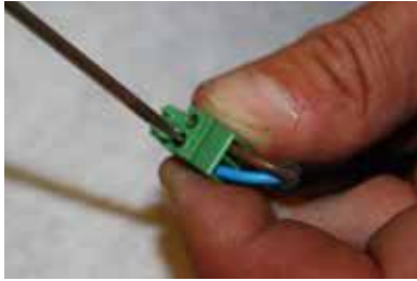
Mount cables and tighten screws
