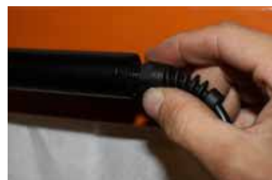
Tighten carefully by hand to make waterproof
