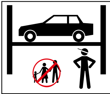
Only authorized persons are allowed to enter the danger zone
