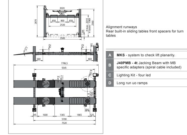
The MKS kit allows to place the four targets and check the perfect lift planarity. Targets, cameras and turn tables are part of the wheel aligner and not included with the lift.
