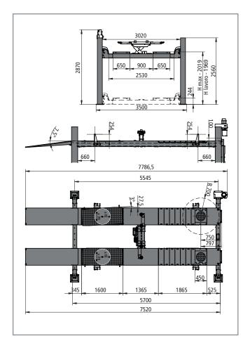
Alignment runways Rear built-in sliding tables front spacers for turn tables
