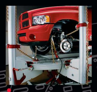
Simultaneous mulitiple pulling capability to precisely reverse damage for faster, higher quality repairs.
