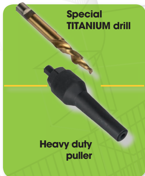
Glow plug remover and repair set for M8, M9, M10
