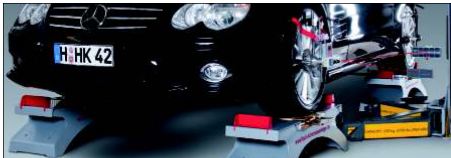
Measurement together with a two-post-lift
