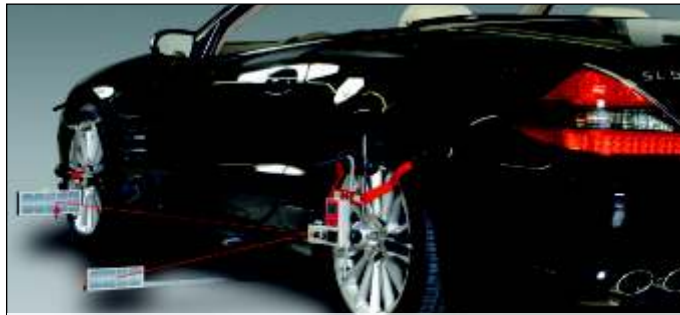
Rear axle measurement with the HD-10 EasyTouch
