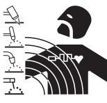
Electric current following through any conductor causes localized Electric and Magnetic Fields (EMF). Welding/cutting current creates EMF fields around cables and power sources.
