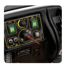
User friendly analogic control panel. Control lever for brush operation and detergent water outflow. ON/OFF and battery cutout key switch, brush and vacuum motor switch, detergent dosing knob (optional), Thermal circuit breaker to protect vacuum and brush motor, battery level indicator, hour meter (optional).
