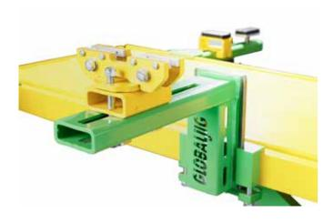
With the wide and fast height adjustment of the sill clamps it is possible to fix and lock any type of vehicle that has the edges of the crests from a minimum 89 mm to a maximum of 308 mm and it is therefore possible to apply and use on the bench any type of system computerized electronic measurement.
