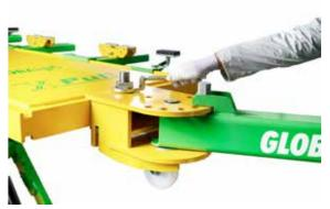
The pull arm is powerful and removable, it is applicable at any point of the frame, with the special key supplied you get a quick and secure tightening, to pull and straighten cars in any 360° direction.
