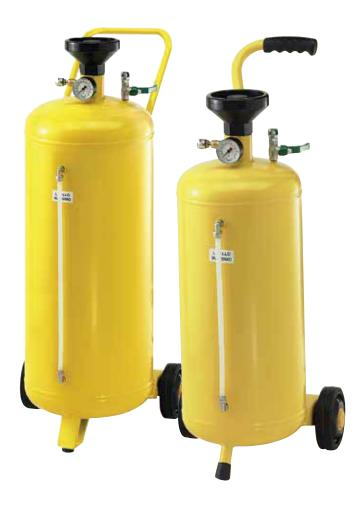
Pneumatic charge sprayers need to be connected to an air compressor to charge the tank and allow the product vaporization without the connection to the air compressor. They work at high-pressures and so they use capacious steel or stainless steel tanks to allow a greater working autonomy.
