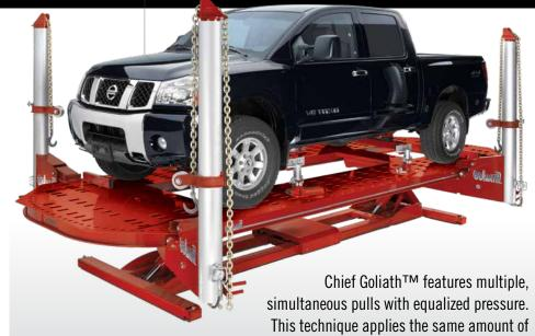
pressure across multiple points of the damaged area at the exact same time, to prevent ripping, tearing, bending or rolling of high-strength steel. Pulling a single area at a time or pulling multiple areas without equalized pressure can actually put more damage into a vehicle. These Chief pulling systems also supply 10 tons of pulling power at the hook. Other systems may use 10-ton rams, but by the time the pressure gets to the hook, the pressure could have dropped to as little as four tons.
