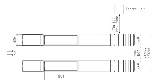
x) Recommended distance (with scissor jack = 875mm)xx) Recommended distance (with scissor jack = 2195mm)
