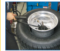
G1001.24AXIT G1005.ELIT Версии с бескамерной накачкой шин. Versions with tubeless tyre inflation system.
