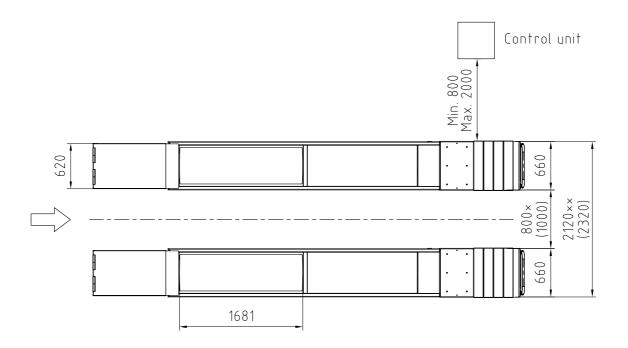
x) Recommended distance (with scissor jack = 875mm)xx) Recommended distance (with scissor jack = 2195mm)
